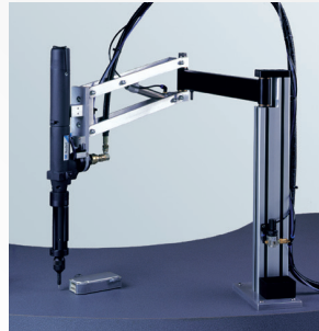
Single-head workstations provide rapid assembly, making them cost effective even with small batch sizes. Available as pantograph, fixed arm or under bench workstation.
