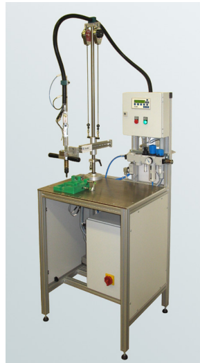
Speed Fastening® module with rivet process monitoring and release function at balancer arm for assembly of AC converter.
