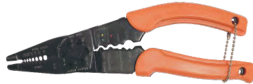
20716 Multi-Function Crimping Tool Cuts/Strips/Crimps 22-10 ga. Non and Insulated Terminals, Flag Terminals, Bolts, W/ Pliar Tip and Spring Loaded Handle Length 8-5/8"
