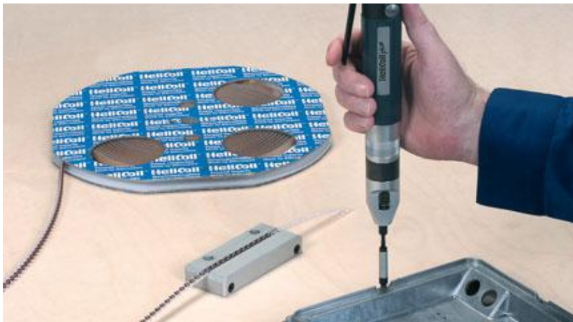
Installation of HELICOIL® Plus
