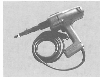
C-410 (for medium production) Electrically-operated, pistol grip header for medium production.
